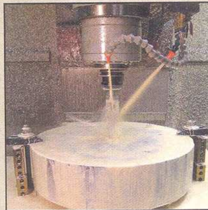
After the first two operations, the blank is secured in the FV-40 Femco vertical mill for two more operations using 24 different pieces of tooling. This machine cuts the windows and spokes from rough cut to finish cut.
