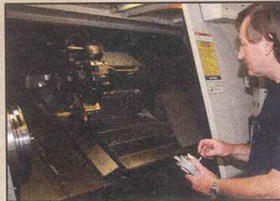
Programming and tooling commands on the Haas SL-40 can be done with the central keypad or this hand-held controller.
