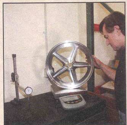
Quality control requires a granite surface table, which is perfectly flat (and level). Here, Tim weighs a dragster front wheel after machining was complete, and it tipped the digital scale at a scant 5.2 pounds. We asked him what other wheels might weigh and Gibson replied, "Between seven and nine pounds." These trick wheels are one-piece, fully machined, with no welding, bolts or rivets.
