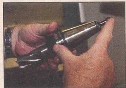
The Femco vertical mill is equipped with Cat 40 tool holders, which were originally designed by the Caterpillar Corporation.
